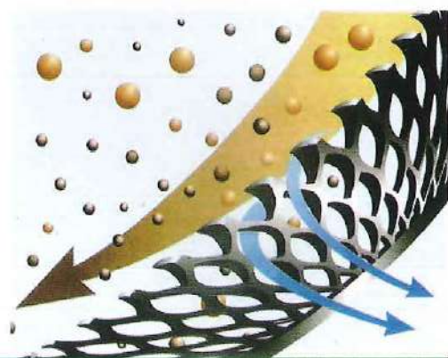
Indirect screening technology Flow tangential to screen retains solids without blinding
