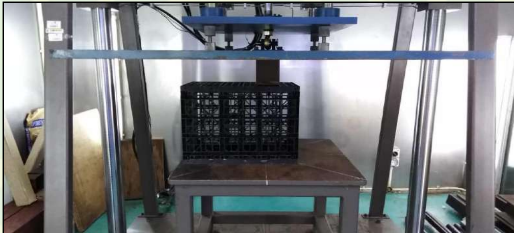
Figure 2: Toughness Test using 120mm x 120mm footprint pad
